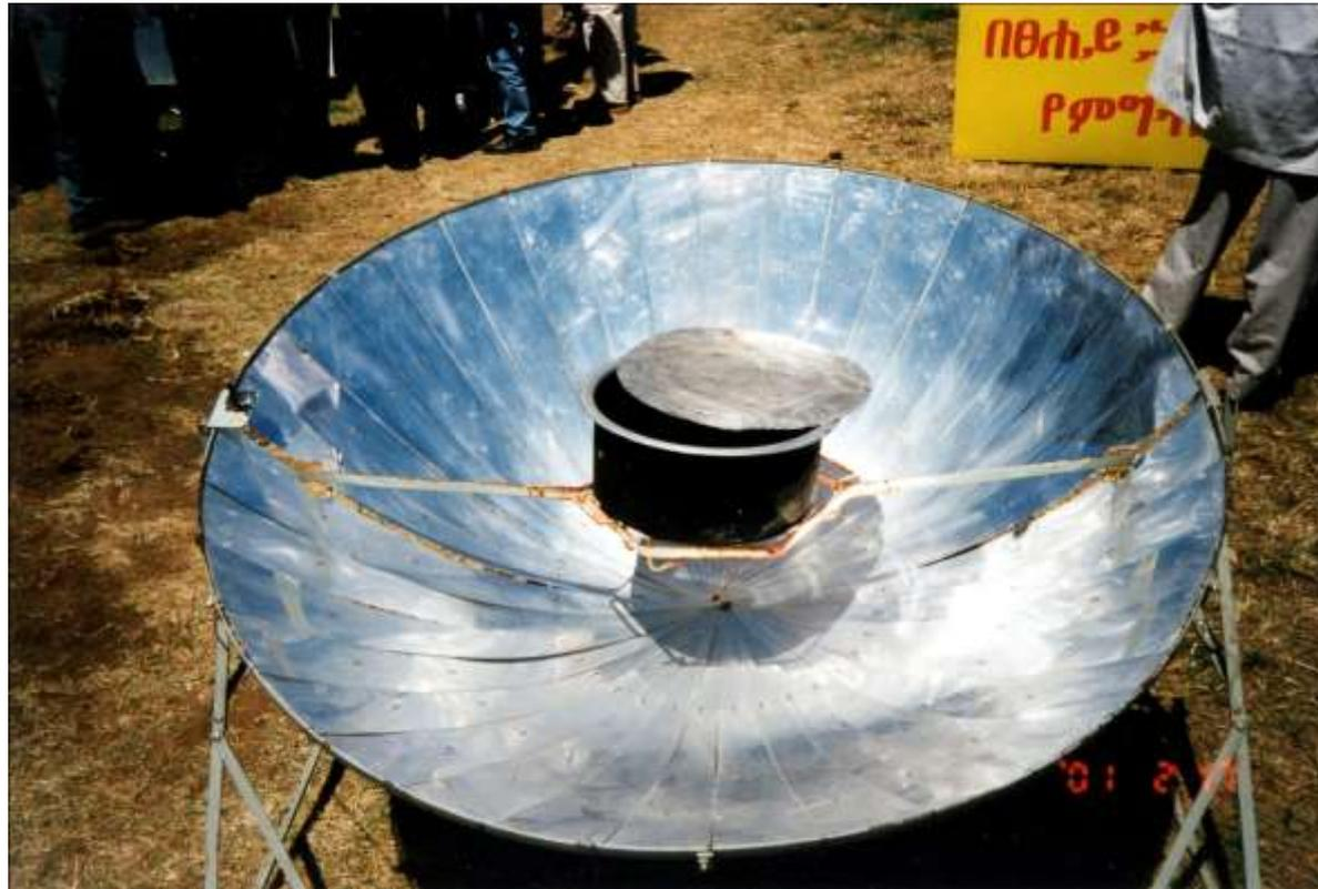
Round parabolic solar grill made from gypsum with sisal fibre, Burayu BTCentre Ethiopia 1982.
